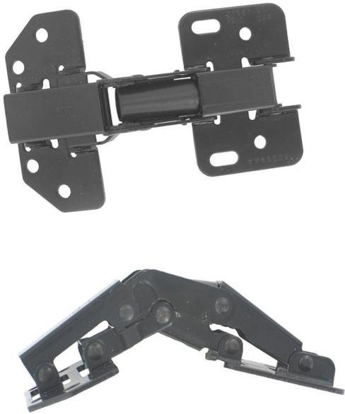
Cabinet hinge is a concealed hinge that surface mounts for ease of installation and totally hidden applications. The concealed hinge action has a rotational axis outside of the physical door (up and out) and provides for flush doors when closed.
